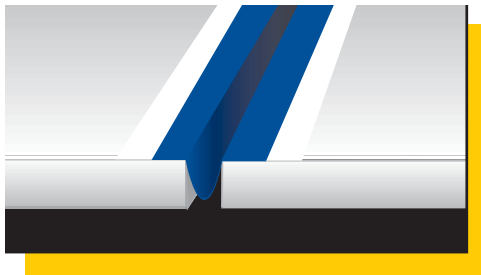
positioning of Mapeband inside an expansion joint
